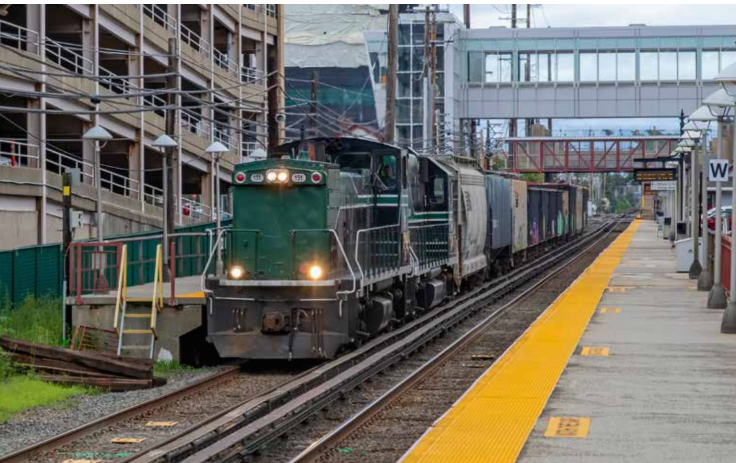
RS-41, the westbound leg of the New York & Atlantic's regular daytime train on the LIRR Main Line, passes through Mineola, N.Y., on July 23, 2019. End plates and steps must be modified to provide clearance for the third-rail electrification on the Main Line. Charles Freericks
