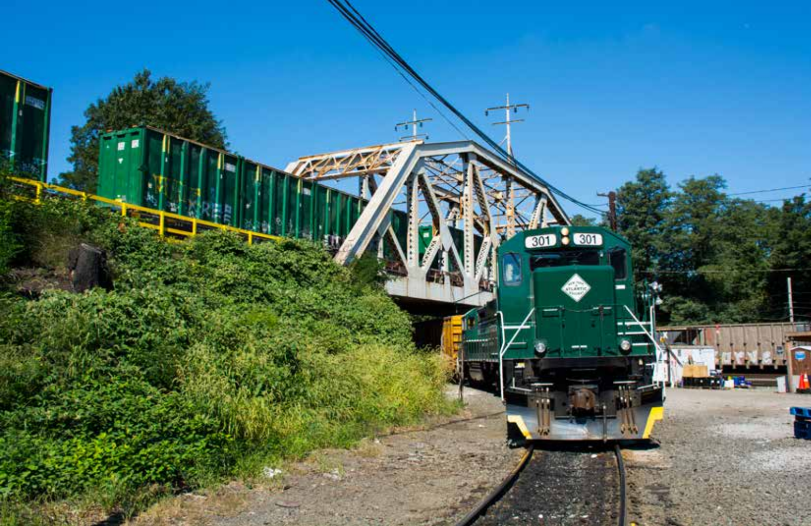
At the NY&A's Fresh Pond Yard, the railroad's PR20Bs wait to take out one train while another crew shoves outbound cars for CSX overhead on Oct. 1, 2017. Tight curves on the wye at Fresh Pond limit the NY&A to four-axle power. Gregory Grice
