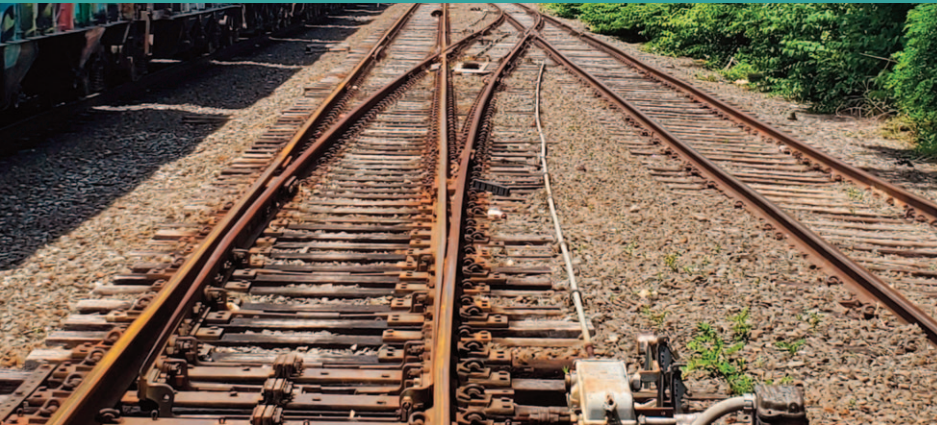
These two unused turnouts in the Fresh Pond West Yard will be moved and placed in the East Yard to improve train movements.
