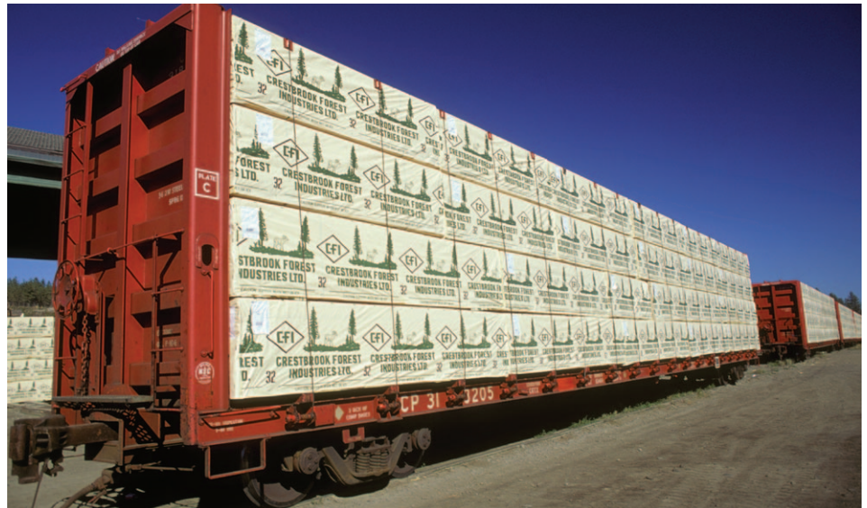
Centerbeam flatcars like this one car carry as many as four truckloads of lumber to the JM Allen transload facility on LIRC.
