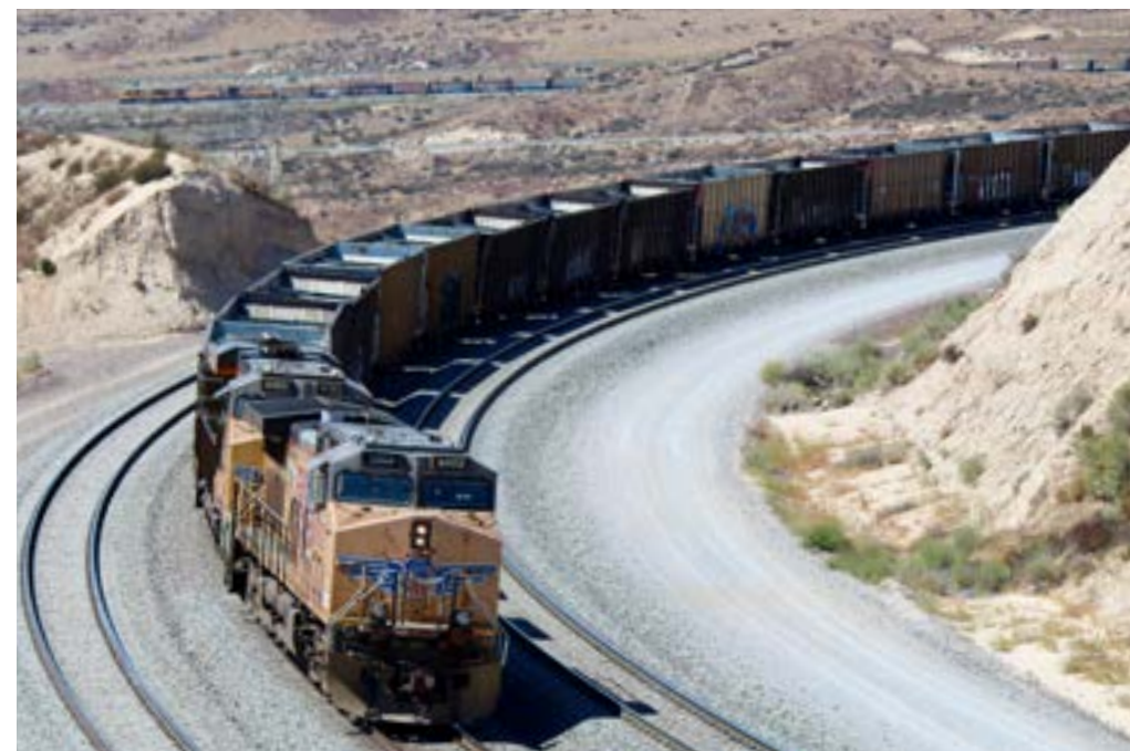
Bound for PHL and an export facility at the Port of Long Beach, 154-car Union Pacific iron ore train OUTSI creeps down Cajon Pass on Sept. 11, 2021, with C45ACCTE No. 6002 as the trailing distributed power unit. The lead locomotives of the 8,174-foot, 21,504-ton train are visible downgrade in the distance.
