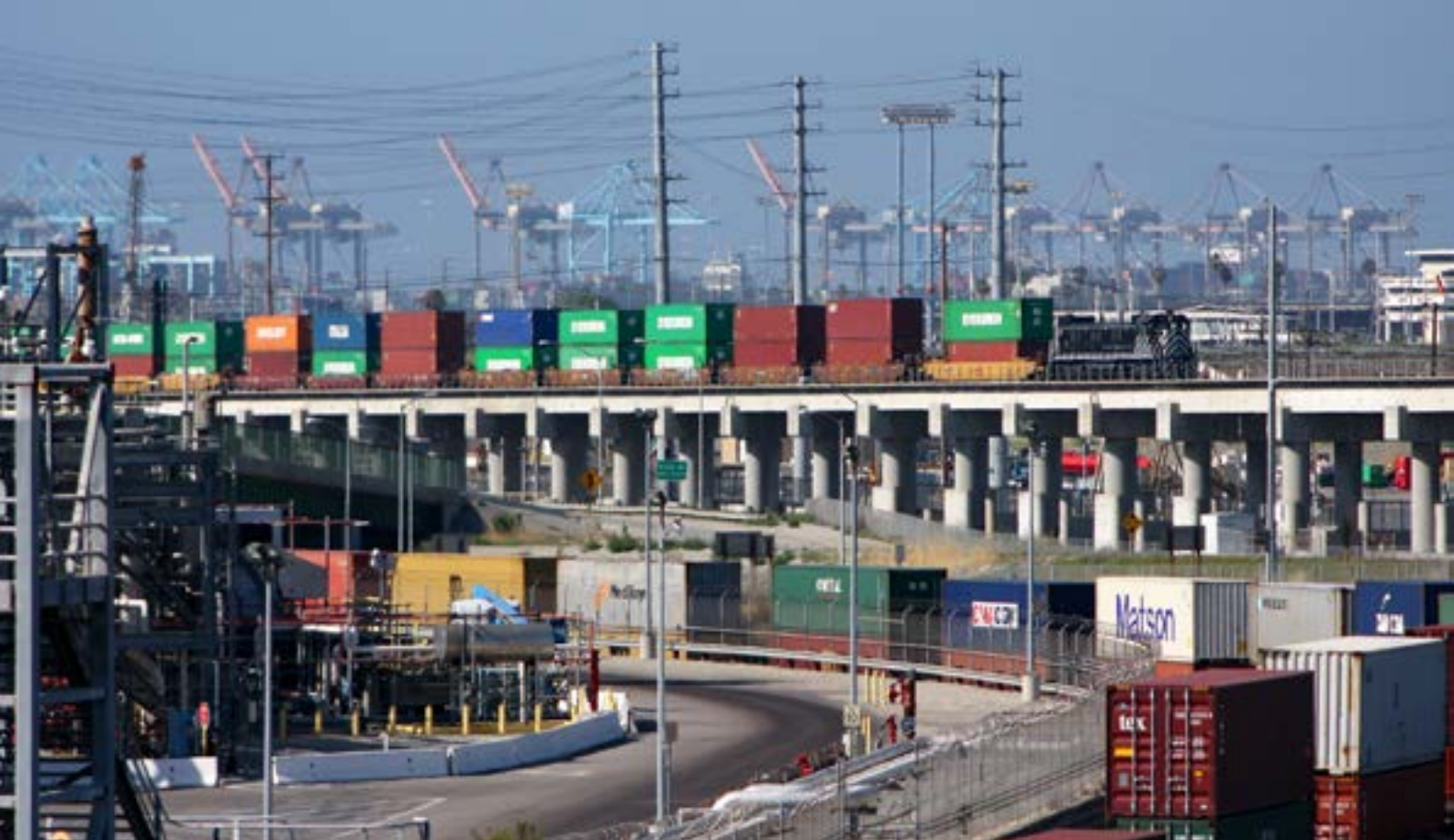
One of Pacific Harbor Line's 3GS21C genset locomotives pulls a long stack train for clearance over Henry Ford Avenue in Wilmington. PHL jobs generally work with a single unit despite the lengthy trains the railroad handles. Two photos, Charles Freericks
