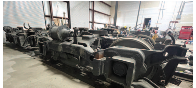
Donated Alco locomotive trucks will keep historic trains rolling for years to come.
