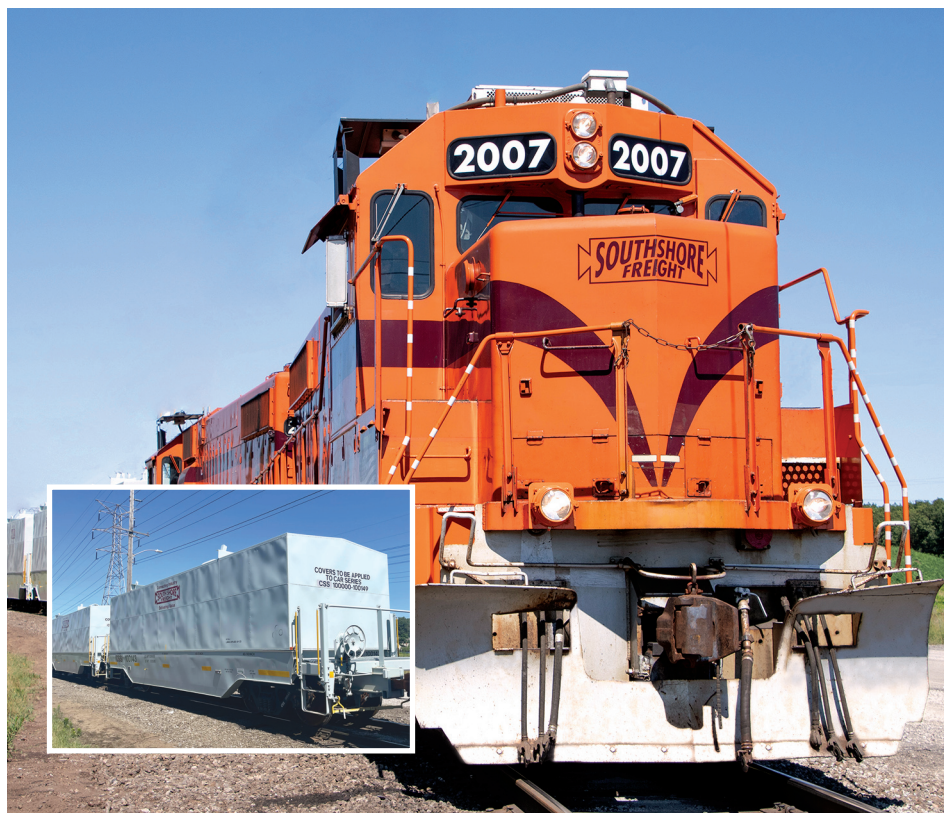
100 new 48-foot, 115-ton-capacity, five-well steel coil cars are being equipped with RailPulse technology.
