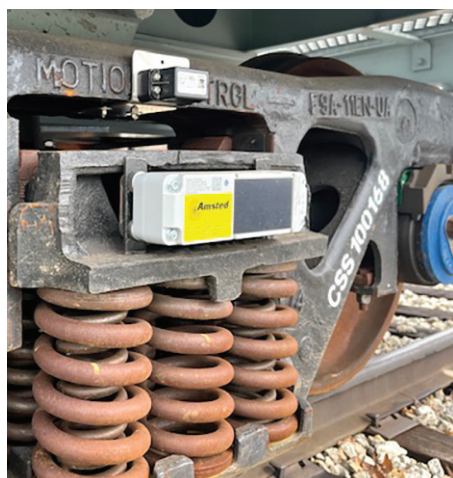
Amsted gateway transmits rail car RailPulse data in real time.
